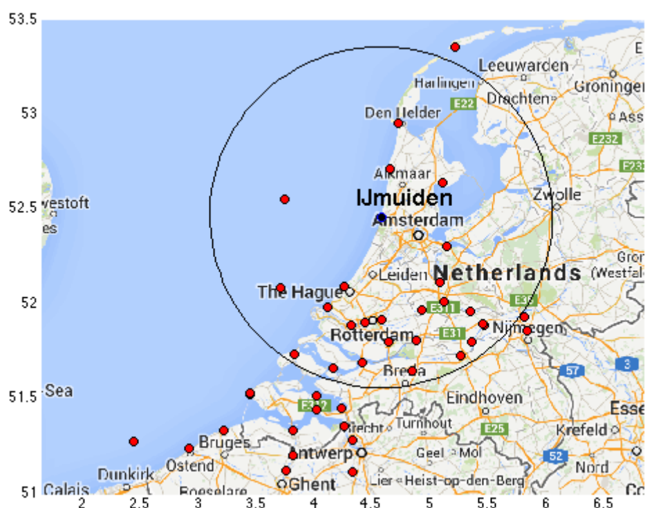
Figure 41: IJmuiden test transmitter with 100km range ring; AIS sites are red dots, MF DGNSS test transmitter is black dot.
